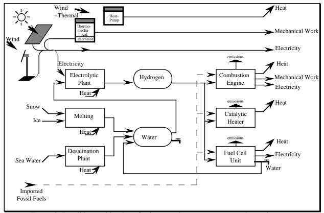
Figure 3: Possible combinations for improved energy systems at the stations.
