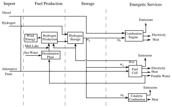
Fig. 2: Alternative Energy System Schematic.
