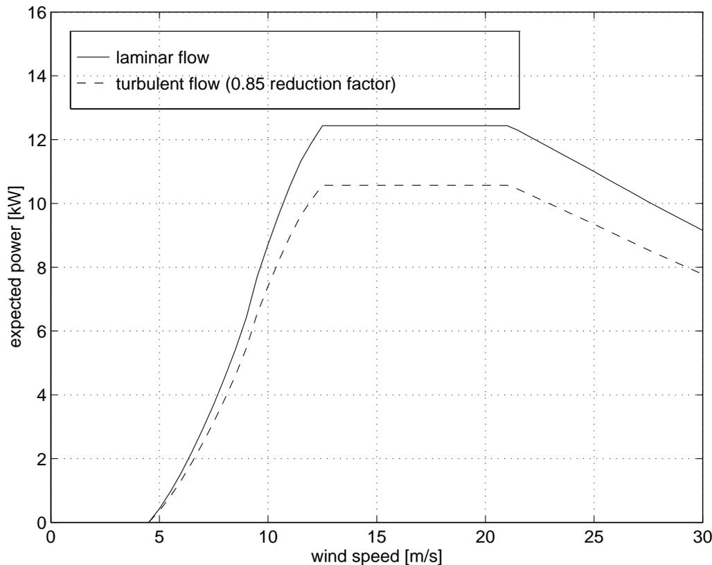
Figure 7: Power curve for UM-70X
