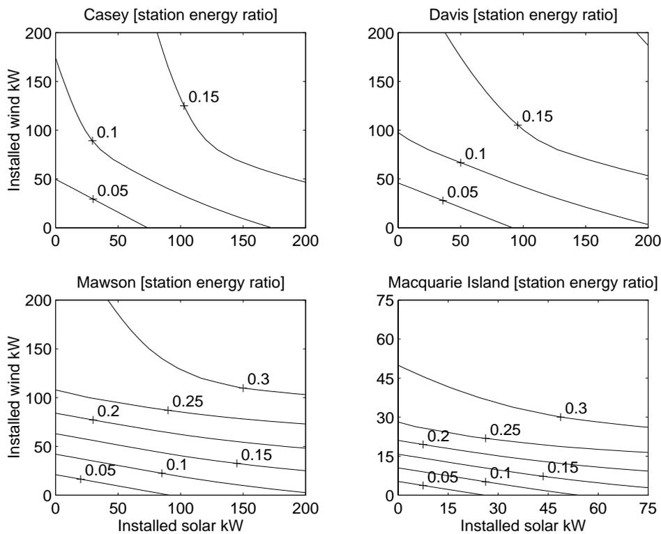
Figure 8: Station energy ratio met by renewables (40% load limit)
