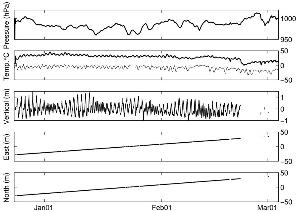
Figure 6: Pressure, temperature and the north, east and vertical components of motion as determined using the GPS data at TS3. The two temperatures shown are the air temperature inside the box (thick line) and the external air temperature measured by the nearby AWS (thin line).
