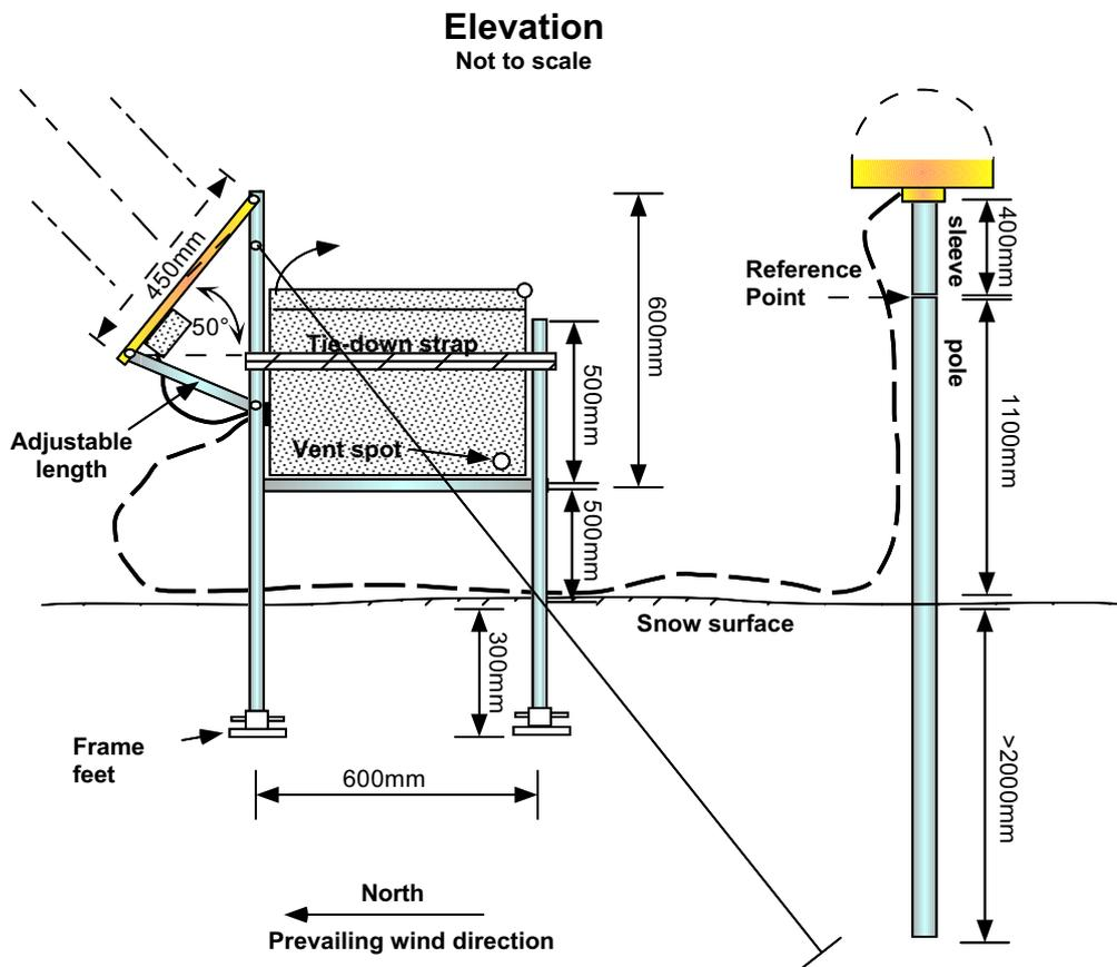
Figure 4: Elevation of the GPS system. Dimensions are approximate and will vary depending on the storage box dimensions
