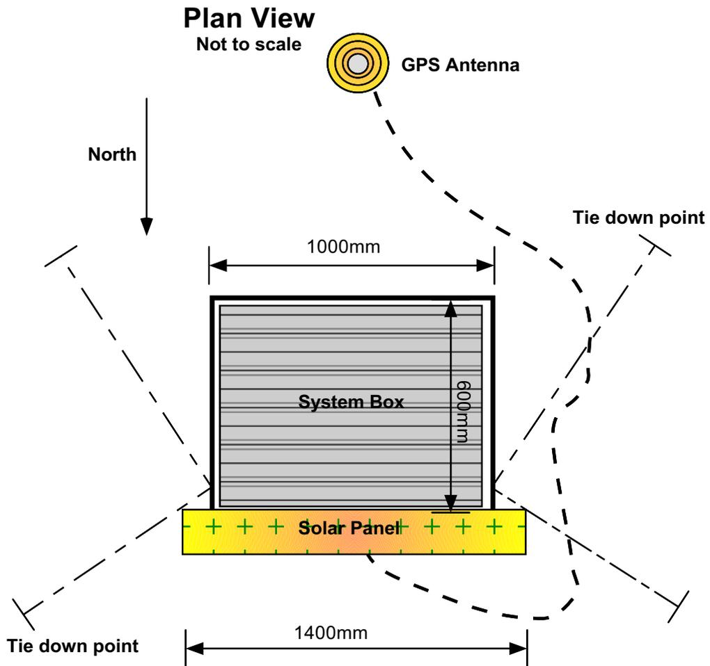
Figure 3: Plan view of the GPS system. Dimensions are approximate and will vary depending on the storage box dimensions.
