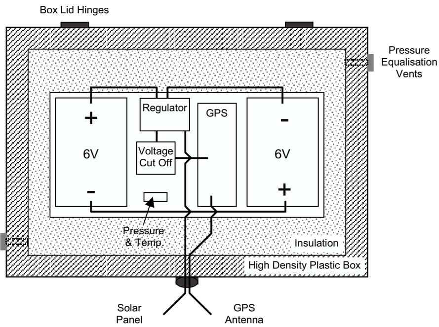
Figure 1: Internal system box components and layout.
