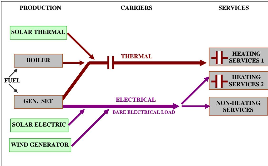
Figure 3: Hybrid system with no diversion capability
