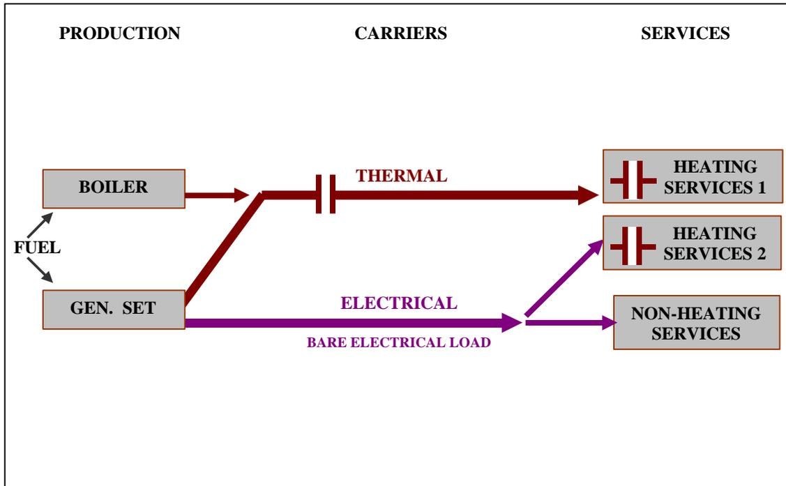
Figure 1: Fossil-fuel based system with no diversion capability
